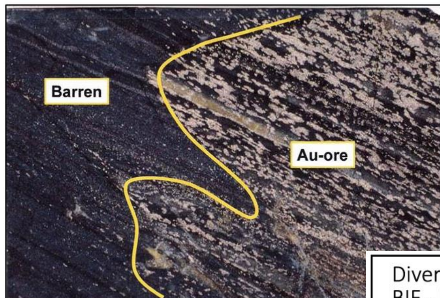
BIF-hosted Gold Deposit: Note fine scale pyrite replacement of magnetite and associated Au ore (photo from David Groves)
